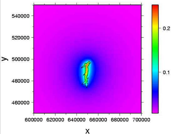
**Figure 4:** The image shows the large scale impact of the Háslón reservoir. It was modeled using a Young's modulus of 50 GPa, a 200 m x 200 m grid, and a water surface at 626 m a.s.l. For this Young's modulus the subsidence exceeds 1 mm within a distance of about 10 km from the reservoir (X and Y coordinates in meters, subsidence in centimeters).
