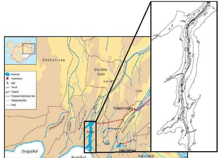
**Figure 1:** Map showing the future location of the reservoir. Close-up shows topography of the reservoir. Steepest parts are in the North. Each contour line represents 25 m elevation difference. (changed from: Landsvirkjun, EIA)
