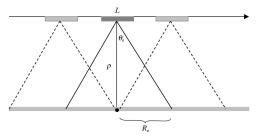
Figure A7. Top view of SAR antenna imaging a point reflector. The reflector remains within the illumination pattern over the real aperture length of  $2R_a$ .
