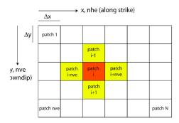
$$I_i = rac{s_{i-nve} - 2s_i + s_{i+nve}}{\Delta x^2} + rac{s_{i-1} - 2s_i + s_{i+1}}{\Delta x^2}$$
