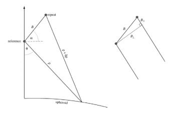
map topography from lat, lon, height to radar coordinates and topography over range, azimuth t(ρ, a)
