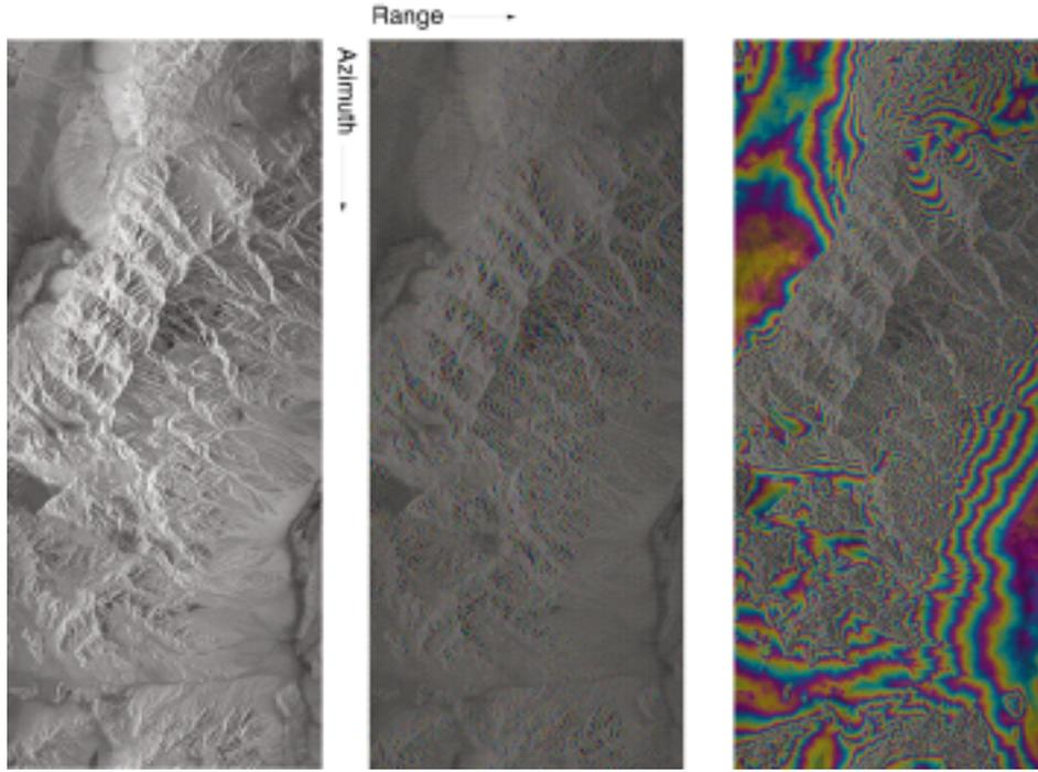
**Fig. 12.** (a) Radar brightness image of Mojave desert near Fort Irwin, CA derived from SIR-C C-band (5.6-cm wavelength) repeat-track data. The image extends about 20 km in range and 50 km in azimuth. (b) Phase of the interferogram of the area showing intrinsic fringe variability. The spatial baseline of the observations is about 70 m perpendicular to the line-of-sight direction. (c) Flattened interferometric phase assuming a reference surface at zero elevation above a spherical earth.
