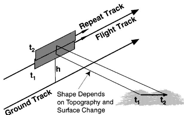
**Fig. 5.** A repeat-track interferometer is similar to an along track interferometer. An aperture repeats its track and precisely measures motion of the surface between observations in the image phase difference. If the track does not repeat at exactly the same location, some topographic phase will also be present, which must be removed by the methods of differential interferometry to isolate the motion.
