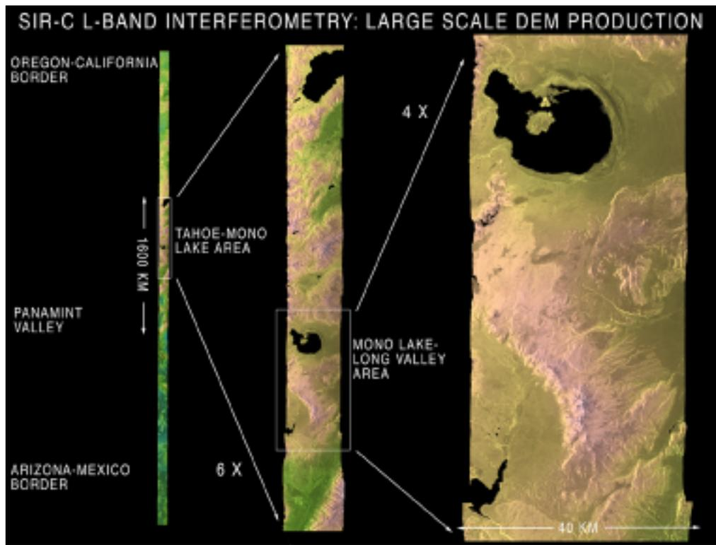
**Fig. 30.** Strip of topography generated from the SIR-C L-band radar data by repeat track interferometry. The DEM extends from the Oregon/California border through California to Mexico, roughly 1600 km.
