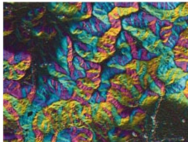
**Fig. 29.** Height (above) and slope (below) maps of Mount Sonoma, CA. This information has been used to assess the risk of earthquake damage induced by landslides. (Processing courtesy E. Chapin, JPL.)
