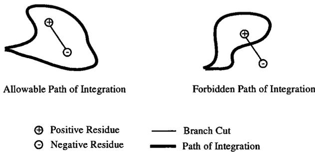
Fig. 18. An example of a branch cut and allowable and forbidden paths of integration.
