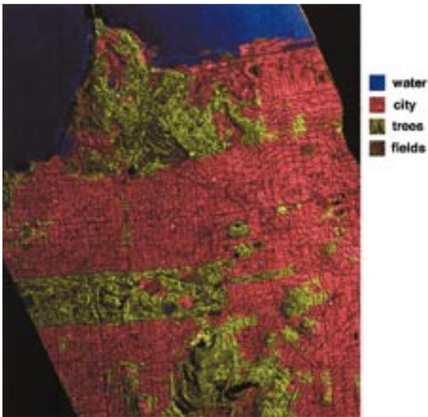
**Fig. 50.** Classification of San Francisco using JPL TOPSAR (C-band) image brightness, interferometric correlation, and topographic height and slope.
