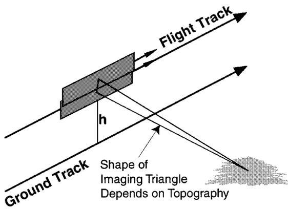
**Fig. 3.** Interferometric SAR for topographic mapping uses two apertures separated by a “baseline” to image the surface. The phase difference between the apertures for each image point, along with the range and knowledge of the baseline, can be used to infer the precise shape of the imaging triangle to derive the topographic height of the image point.
