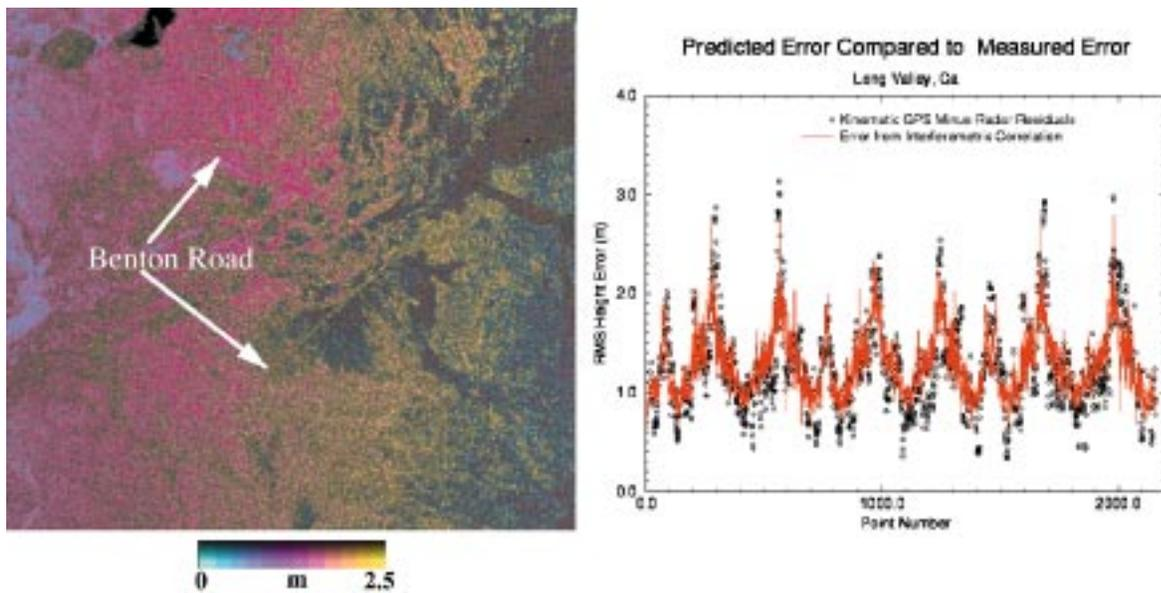
**Fig. 36.** Illustration of the use of kinematic GPS surveys in determining the absolute and relative error of a radar-derived DEM. Curve shows the standard deviation of the radar height relative to the GPS and its predicted value. Statistical height error estimates derived from the correlation track the measured local statistical height errors extremely well.
