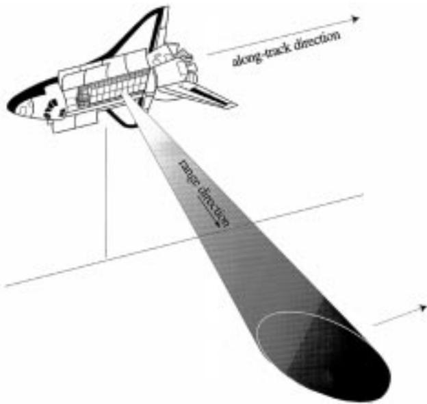
**Fig. 1.** Typical imaging scenario for a SAR system, depicted here as a shuttle-borne radar. The platform carrying the SAR instrument follows a curvilinear track known as the “along-track,” or “azimuth,” direction. The radar antenna points to the side, imaging the terrain below. The distance from the aperture to a target on the surface in the look direction is known as the “range.” The “cross-track,” or range, direction is defined along the range and is terrain dependent.
