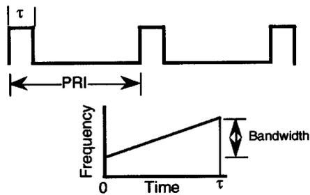
**Fig. 51.** The radar emits a sequence of pulses separated in time. The time duration between pulses is called the inter pulse period (IPP) and the associated pulse frequency is called the pulse repetition frequency (PRF = 1/IPP). The pulse duration is denoted  $\tau$ .
