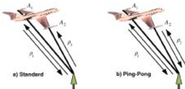
**Fig. 8.** Illustration of standard versus "ping-pong" mode of data collection. In standard mode, the radar transmits a signal out of one of the interferometric antennas only and receives the echoes through both antennas,  $A_1$  and  $A_2$ , simultaneously. In "ping-pong" mode, the radar transmits alternatively out of the top and bottom antennas and receives the radar echo only through the same antenna. Repeat-track interferometers are inherently in "ping-pong" mode.
