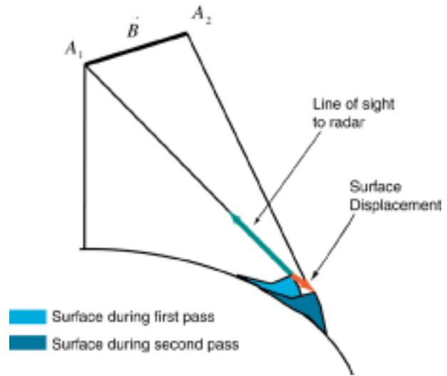
**Fig. 17.** Geometry of displacement interferometry. Surface element has moved in a coherent fashion between the observation made at time  $t_1$  and the observation made at time  $t_2$ . The displacement can be of any sort—continuous or instantaneous, steady or variable—but the detailed scatterer arrangement must be preserved in the interval for coherent observation.
