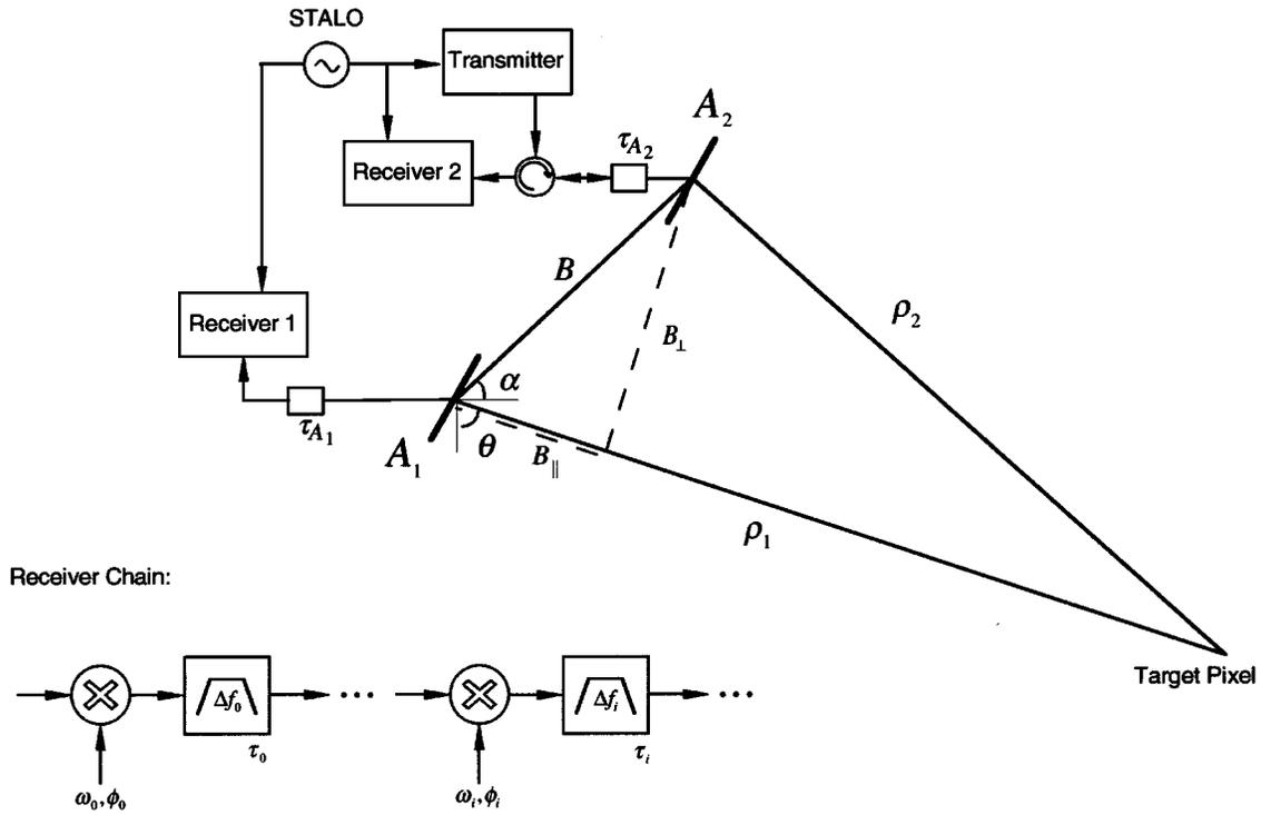
**Fig. 16.** Definitions of interferometric parameters relating to a possible radar interferometer configuration. In this example, the transmitter path is common to both roundtrip signal paths. Therefore the transmitter phase and time delays cancel in the channel difference. The total delay is the sum of the antenna delay and the various receiver delays.
