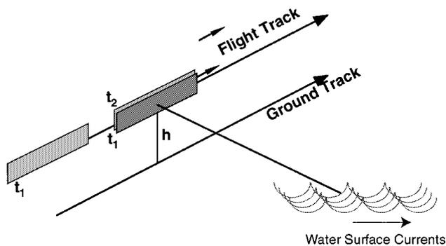
**Fig. 4.** An along-track interferometer maintains a baseline separated along the flight track such that surface points are imaged by each aperture within 1 s. Motion of the surface over the elapsed time is recorded in the phase difference of the pixels.
