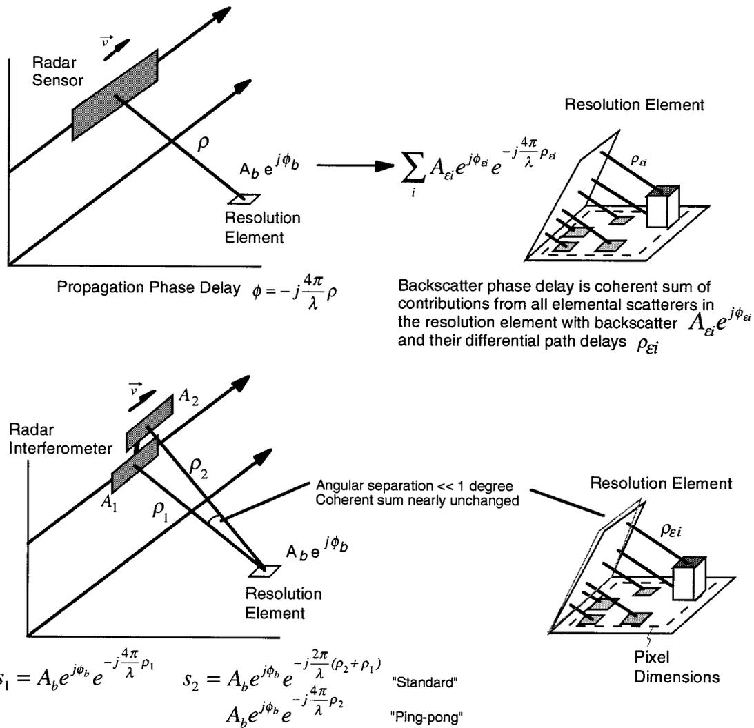
**Fig. 7.** The interferometric phase difference is mostly due to the propagation delay difference. The (nearly) identical coherent phase from the different scatterers inside a resolution cell (mostly) cancels during interferogram formation.
