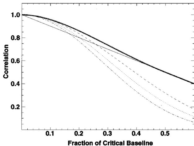
**Fig. 21.** Baseline decorrelation for various point target response functions. The solid line is for standard sinc response with no weighting. The dashed, dotted-dashed, dotted, and triangled lines are weightings of half-cosine, Hanning, Hamming, and optimized cosine, respectively.
