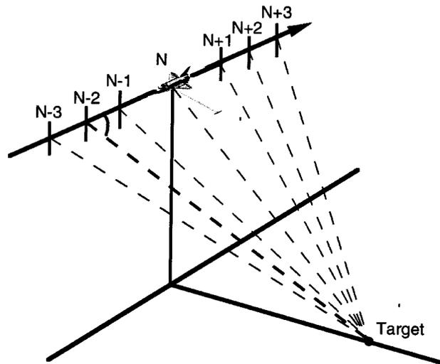
**Fig. 53.** A sensor imaging a fixed point on the ground from a number of pulses in a synthetic aperture. The range at which a target appears in a synthetic aperture image depends on the processing parameters and algorithm used to generate the image. For standard range-Doppler processing, the range is fixed by choosing the pulse that has a user-defined fixed angle between the velocity vector and the line-of-sight vector to the target. This is equivalent to picking the Doppler frequency.
