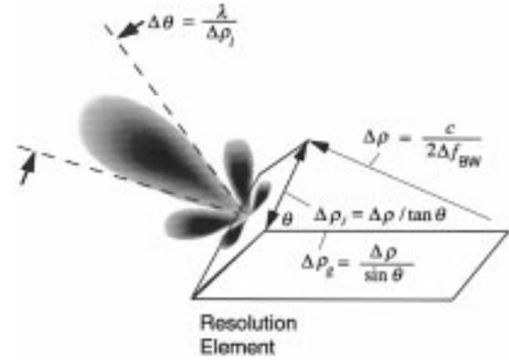
**Fig. 20.** A view of baseline decorrelation showing the effective beam pattern of a ground resolution element “radiating” to space. The mutual coherence field propagates with radiation beamwidth in elevation of  $\Delta\theta \approx \lambda/\Delta\rho_l$ . These quantities are defined in the figure.
